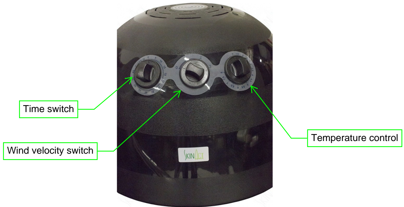
Control panel (Time, Wind Velocity, and Temperature dials)
